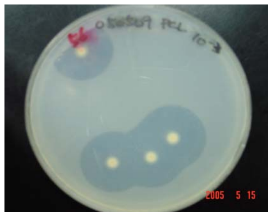
Fig. 9 The colonies and clear-zone formation by strain HS 45-1 on agar plate with emulsified PCL-agar plate at 50 °C
